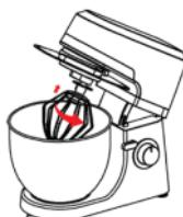
8. Gently press the front head and then press release button to release the head and raise it to a vertical position.
