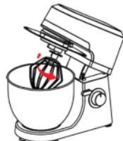
10. Fit the desired attachment into the attachment slot, pushing the shaft of the accessory into the slot and turn it in clockwise/anticlockwise direction until it clicks into place.
